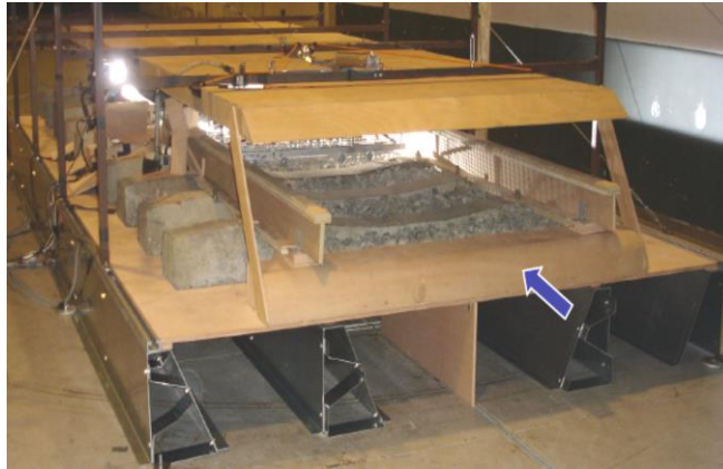
Fig 13 Wind tunnel tests on full scale track bed (36)
