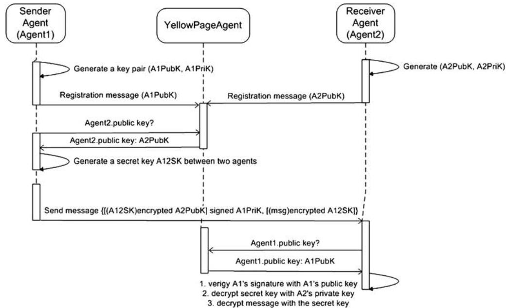
**Figure 4** The sequence diagram of secure message transportation
