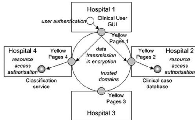
**Figure 2** Overview of the security model layers using a cross-hospital resource access scenario
