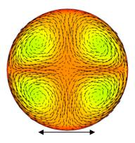
Figure 11: Velocity vector plot superimposed on temperature distribution across the oscillated pipe.
