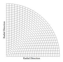
Figure 2: Illustration of grid used for evaluation of volume-flowrate weighted mean temperature and area-weighted pressure over pipe section (total number of cells, *N* = 1860 cells).
