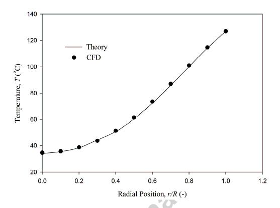
Figure 6: Comparison of CFD-predicted and theoretical (Eq. 14) axial temperature profiles for isoviscous non-Newtonian power law fluid in steady laminar pipe flow:  $T_{in} = 27$  °C;  $T_{w} = 127$  °C; D = 30 mm;  $\overline{w} = 1.0$  cm s<sup>-1</sup>;  $\rho = 998$  kg m<sup>-3</sup>; k = 1 Pa s<sup>0.5</sup>; n = 0.5;  $C_{p} = 4180$  J kg<sup>-1</sup> K<sup>-1</sup>;  $\lambda = 0.6$  W m<sup>-1</sup> K<sup>-1</sup>.
