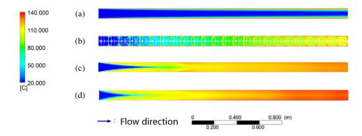
Figure 13: Development of azimuthally-averaged temperature profile along the pipe: (a) simple steady flow; (b) steady flow through helical static mixer; (c) flow with transverse oscillations; (d) flow with transverse oscillations and step rotation of vibration orientation.
