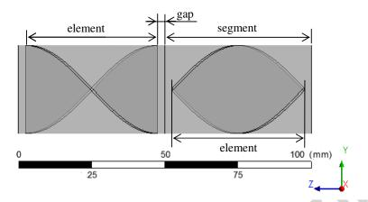
Figure 3: Geometry of helical Kenics static mixer showing two adjacent mixer segments.
