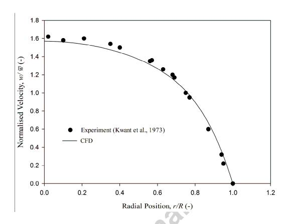
Figure 7: Comparison of CFD-predicted and experimental velocity profiles for a temperature-dependent Newtonian fluid in steady pipe flow with heat transfer:  $T_{in} = 27$  °C;  $T_{w} = 127$  °C; D = 30 mm;  $\overline{w} = 2.0$  cm s<sup>-1</sup>;  $\mu = 1.3$ exp[(T - 25 °C)/ $(T_{w} - T_{in})$ ] Pa s;  $\rho = 998$  kg m<sup>-3</sup>;  $C_{p} = 4180$  J kg<sup>-1</sup> K<sup>-1</sup>;  $\lambda = 0.6$  W m<sup>-1</sup> K<sup>-1</sup>.
