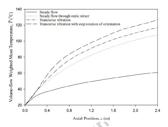
Figure 14: Mean temperature development along the pipe:  $T_{in} = 20$  °C;  $T_w = 140$  °C; D = 30 mm; L = 2400 mm;  $\overline{w} = 4.0$  cm s<sup>-1</sup>;  $\mu = k_0 \exp(E_a/R_gT)$  Pa s;  $\rho = 998$  kg m<sup>-3</sup>;  $C_p = 4180$  J kg<sup>-1</sup> K<sup>-1</sup>;  $\lambda = 0.668$  W m<sup>-1</sup> K<sup>-1</sup>; A = 2 mm; f = 50 Hz.
