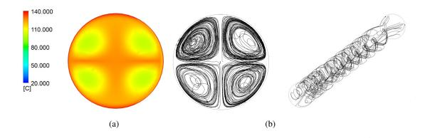
Figure 10: Viscous flow of a temperature-dependent Newtonian fluid in a straight pipe subjected to transverse oscillations: (b) temperature distribution at pipe exit; (b) fluid trajectories.
