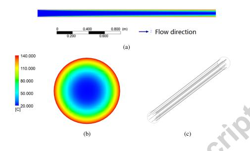
Figure 8: Steady viscous flow of a temperature-dependent Newtonian fluid in a straight pipe: (a) temperature distribution along the pipe; (b) temperature distribution at pipe exit; (c) fluid streamlines.
