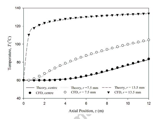
Figure 5: Comparison of CFD-predicted and theoretical (Eq. 14) axial temperature profiles at three different radial positions for isoviscous Newtonian fluid in steady laminar pipe flow:  $T_{in} = 60$  °C;  $T_w = 140$  °C; D = 30 mm;  $\overline{w} = 4.0$  cm s<sup>-1</sup>;  $\mu = 0.001$  Pa s;  $\rho = 998$  kg m<sup>-3</sup>;  $C_p = 4180$  J kg<sup>-1</sup> K<sup>-1</sup>;  $\lambda = 0.6$  W m<sup>-1</sup> K<sup>-1</sup>.
