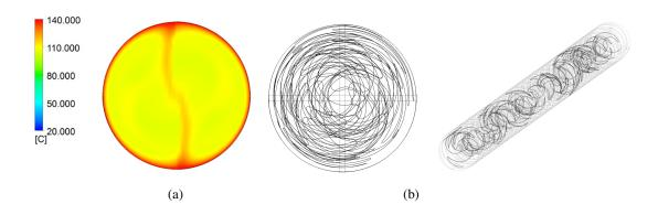
Figure 9: Viscous flow of a temperature-dependent Newtonian fluid in a straight pipe fitted with a Kenics static mixer: (a) temperature distribution at pipe exit; (b) fluid trajectories.
