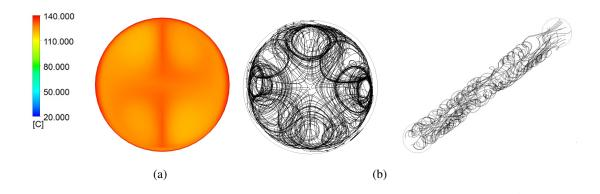
Figure 12: Viscous flow of a temperature-dependent Newtonian fluid in a straight pipe subjected to transverse oscillations with a superimposed step rotation of vibration orientation: (a) temperature distribution at pipe exit; (b) fluid trajectories.
