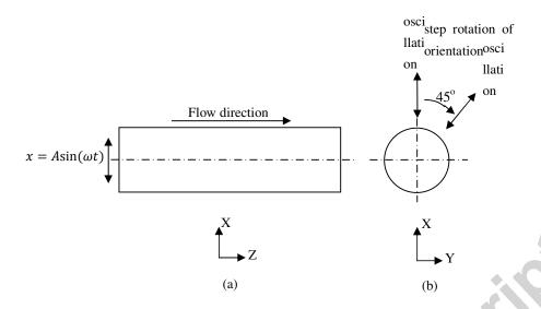
Figure 1: Viscous flow in a straight pipe: (a) under transverse vibration; (b) under transverse vibration coupled with superimposed 45-degree step rotation of vibration orientation.
