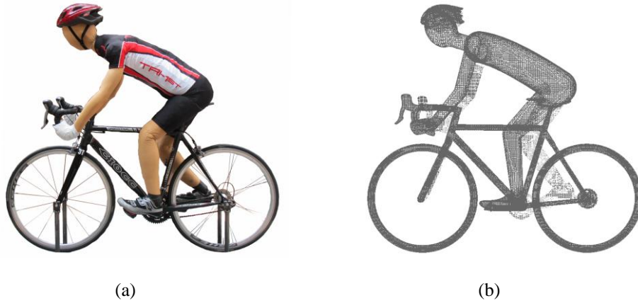
114 Fig. 2: (a) Full-scale bicycle and mannequin used in wind tunnel experiments and (b) geometry of the 115 bicycle and cyclist in simulations.
