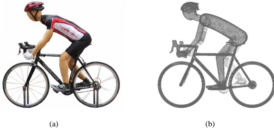
Fig. 2: (a) Full-scale bicycle and mannequin used in wind tunnel experiments and (b) geometry of the bicycle and cyclist in simulations.
