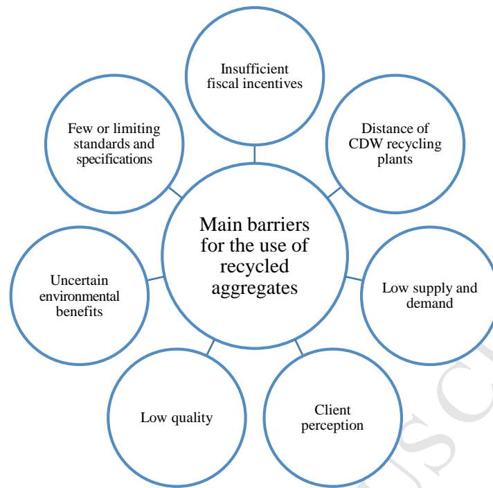
Figure 1 - Main barriers that prevent a wider use of recycled aggregates in construction
