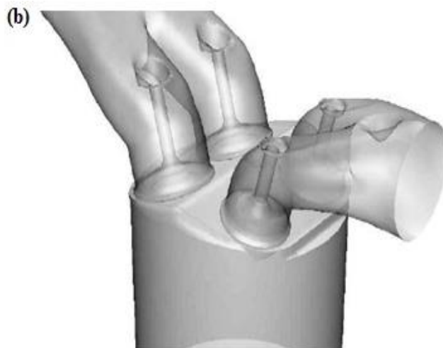
Figure 2 (a) Schematic of Engine and Instrumentation Setup (b) 3D Cylinder Head Diagram
