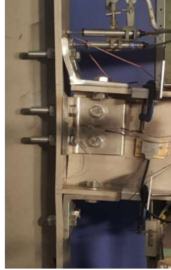
(b) Top and Seat Angle Cleat (TSAC-10) connection failure mode and bolt failure in tension and shear
