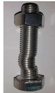
(b) Top and Seat Angle Cleat (TSAC-10) connection failure mode and bolt failure in tension and shear
