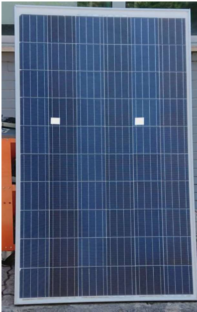
346 347 Fig. 11. The 60-cells module adopted for experiments. 348 Second case test set-up: partially shaded solar cells belonging 349 to different sub-modules. The cell on the left is protected by 350 the standard bypass diode, the cell on the right by the new 351 bypass circuit. 352
