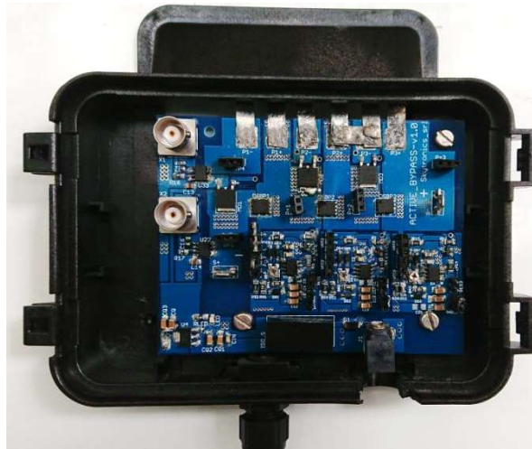
Fig. 5. Rear side photovoltaic module junction box containing three bypass circuits. In the periphery the board contains additional circuits for sensing purposes.
