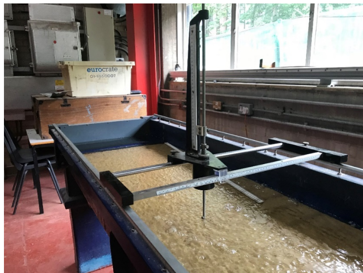
Figure 3 Water accumulated on top of the sand bed
