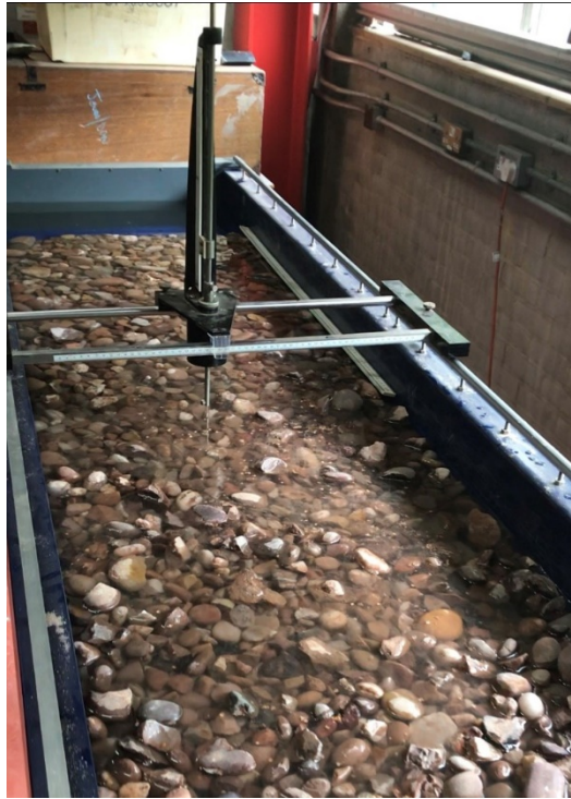
Figure 4 Water accumulated on top of the gravel bed
