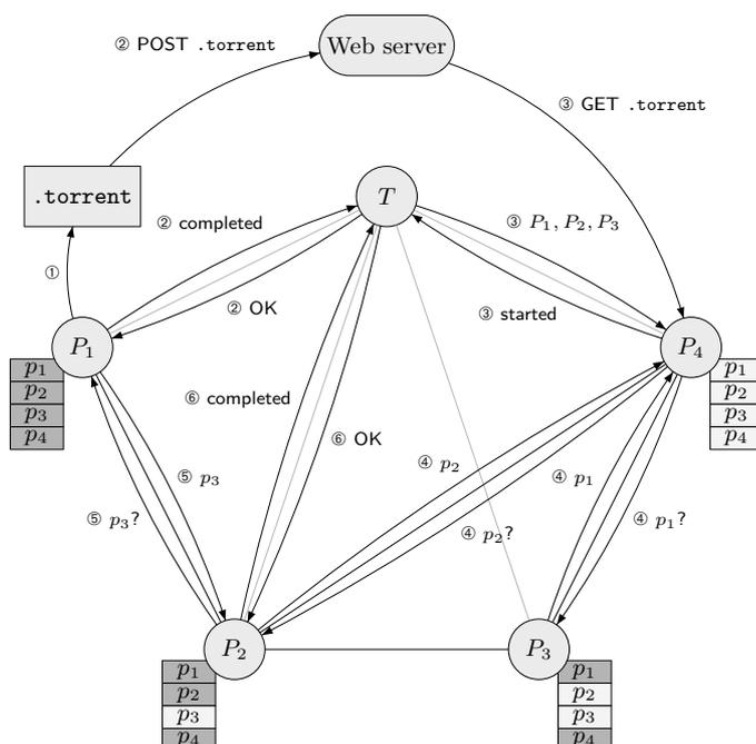
**Fig. 2.** A file being shared using BitTorrent.
