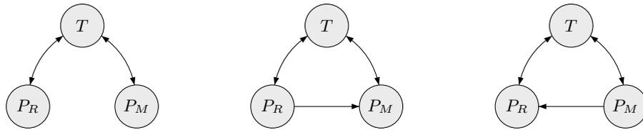
**Fig. 1.** Different methods by which a monitoring peer ( $P_M$ ) may monitor a regular peer ( $P_R$ ) via a tracker ( $T$ ). From left to right: indirect monitoring; passive direct monitoring; active direct monitoring.
