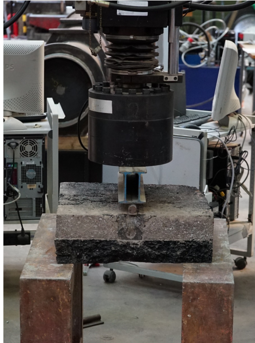
Figure 1: Crack simulation process using an actuator
