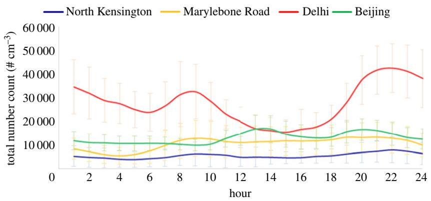
**Figure 2.** Average diurnal variation of particle number counts at the sites in London (North Kensington and Marylebone Road), Beijing and Delhi. The error bars represent one standard deviation. (Online version in colour.)
