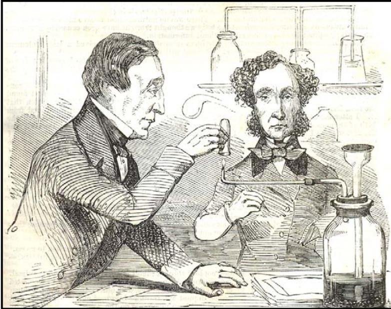
Dr Alfred Swaine Taylor and Dr Rees conducting analyses, and detecting antimony but not strychnine. The apparatus is probably generating hydrogen from zinc granules and sulfuric acid in a form of Marsh's test to detect arsenic and antimony. [From reference 3].
