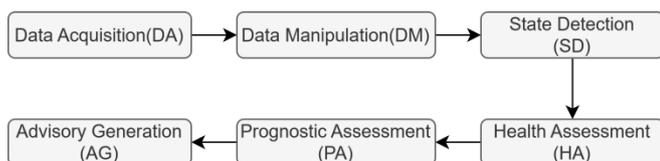
Figure 1: The six processing levels of ISO 13374. Source: [14].
