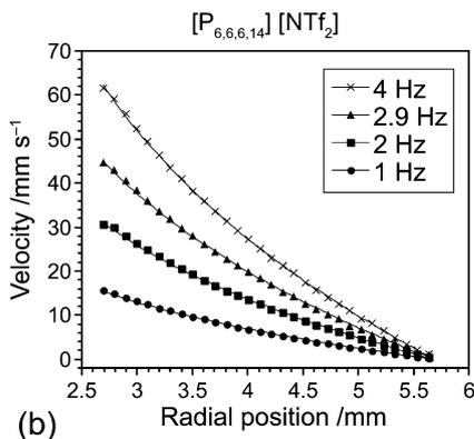
**Fig. 3** Radial velocity profiles taken across the cylindrical Couette cell for neat  $[C_4mim][BF_4]$  (a) and  $[P_{6,6,6,14}][NTf_2]$  (b) ionic liquids at rotation rates of  $\omega = 1, 2, 2.9$  and  $4$  Hz. The line shows the fit obtained using eqn (2), which yielded a value of  $n = 1$  (Newtonian behaviour) in both cases.
