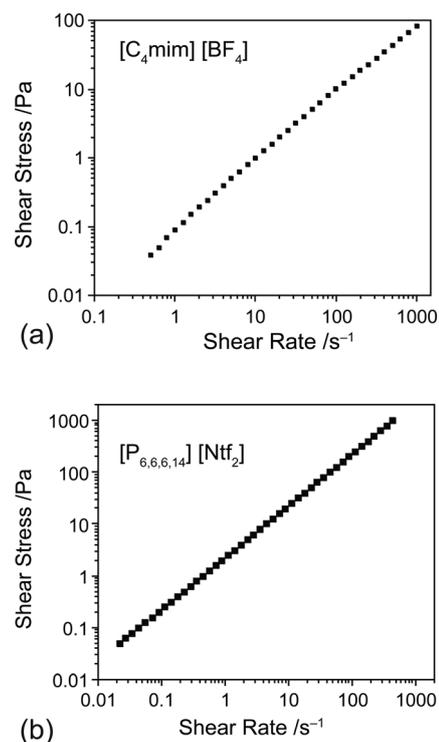
**Fig. 2** Flow curves, showing shear stress as a function of shear rate, for neat  $[\text{C}_4\text{mim}][\text{BF}_4]$  (a) and  $[\text{P}_{6,6,6,14}][\text{NTf}_2]$  (b) ionic liquids.
