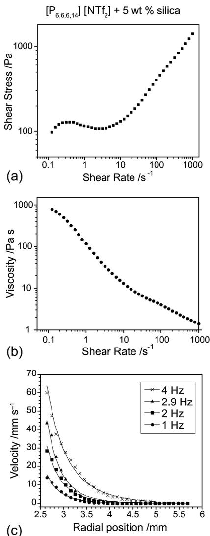
**Fig. 5** Flow curve (a), plot of viscosity vs. shear rate (b) and radial velocity profiles in a Couette cell (c) for  $[P_{6,6,6,14}][NTf_2]$  with 5% w/w Aerosil 200. The line in (c) shows the fit obtained using eqn (2), which yielded values of  $n = 0.20$  at 1 Hz,  $n = 0.21$  at 2 Hz,  $n = 0.28$  at 2.9 Hz and  $n = 0.21$  at 4 Hz.
