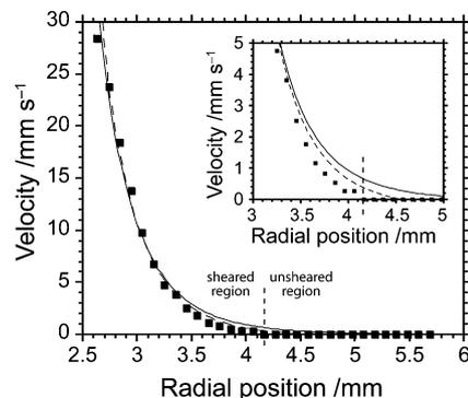
**Fig. 6** Radial velocity profiles taken across the cylindrical Couette cell for  $[P_{6,6,6,14}][NTf_2]$  with 5% w/w Aerosil 200 at a rotation rate of  $\omega = 2 \text{ Hz}$ . The inset plot shows the region by the interface at an expanded scale. The solid line is the fit to eqn (2) with  $r_o$  fixed and  $n = 0.21$  and the dashed line is the fit with  $r_o$  as a fitting parameter with  $r_o = 4.54 \text{ mm}$  and  $n = 0.21$ .
