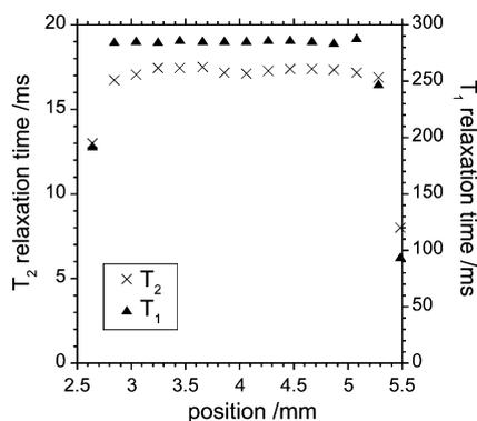
**Fig. 7** Azimuthally averaged  $T_1$  and  $T_2$  magnetic resonance relaxation time profiles through the annulus of a Couette cell for  $[P_{6,6,6,14}][NTf_2]$  with 5% w/w Aerosil 200 at  $\omega = 1$  Hz.
