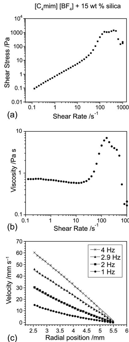
**Fig. 4** Flow curve (a), plot of viscosity vs. shear rate (b) and radial velocity profiles in a Couette cell (c) for  $[C_4mim][BF_4]$  with 15% w/w Aerosil 200. The line in (c) shows the fit obtained using eqn (2), which yielded values of  $n = 1.01$  at 1 Hz,  $n = 1.22$  at 2 Hz,  $n = 2.04$  at 2.9 Hz and  $n = 2.67$  at 4 Hz.
