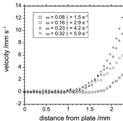
**Fig. 9** Velocity profiles through the gap of a cone-and-plate rheometer for a suspension of  $[P_{6,6,6,14}][NTf_2]$  + 5% w/w Aerosil 200, at a range of rotation rates, from the data shown in Fig. 8. Each profile was taken at a position of 6.56 mm from the tip of the cone, as indicated by the arrow in Fig. 8.
