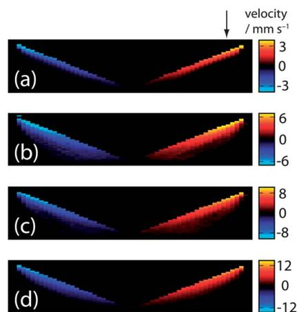
**Fig. 8** Magnetic resonance velocity images for  $[P_{6,6,6,14}][NTf_2]$  with 5% w/w Aerosil 200 in a cone-and-plate rheometer at rotation rates of (a) 0.08 Hz, (b) 0.16 Hz, (c) 0.23 Hz and (d) 0.32 Hz. The displayed field of view is 3.5 mm in the vertical direction and 20 mm in the horizontal direction, with a pixel size of 0.070 mm (vertical)  $\times$  0.313 mm (horizontal). The arrow indicates the position where velocity profiles were taken through the gap of the cone and plate in Fig. 9.
