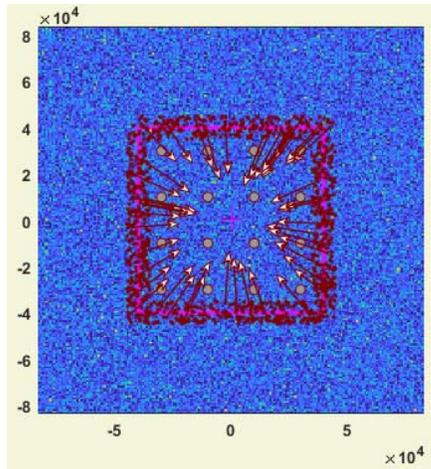
**Fig. 5.** Sonobuoy scenario, with 16 sonobuoys (grey circles) laid out in a grid spaced 20 km apart. The red dots show sample target trajectories, starting in the neighbourhood of the boundary of the operational area and moving towards the centre. The pink square shows  $A_0$ , the area of interest, which is a square area from  $(-40, -40)$  km to  $(40, 40)$  km.
