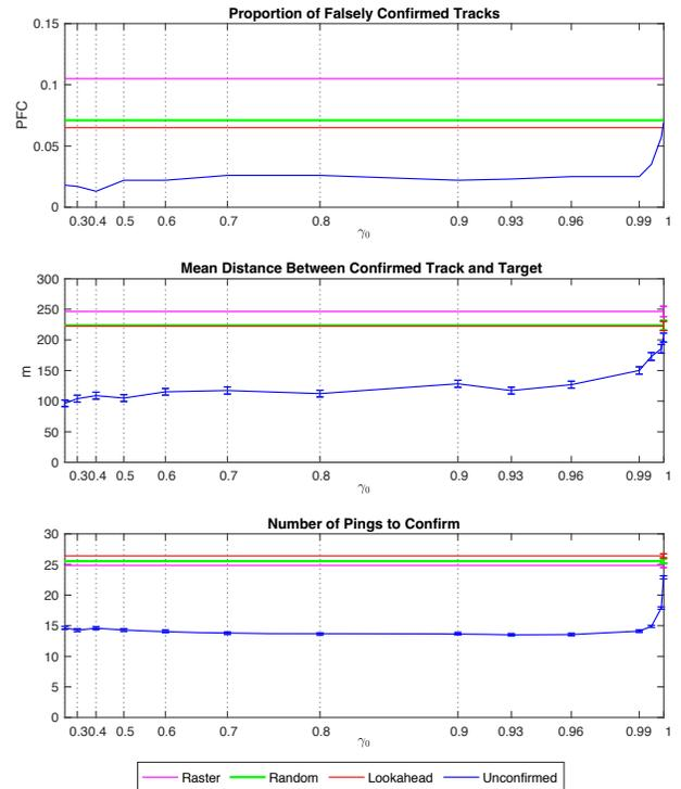
**Fig. 6.** Simulation results, showing the proportion of falsely confirmed tracks, mean distance between the confirmed track and the true target and the number of pings to confirm a target for the 4 methods. Performance is shown for a range of  $\gamma_0$  values, with Unconfirmed being the only method that depends on this parameter. The error bars show plus or minus one standard deviation.
