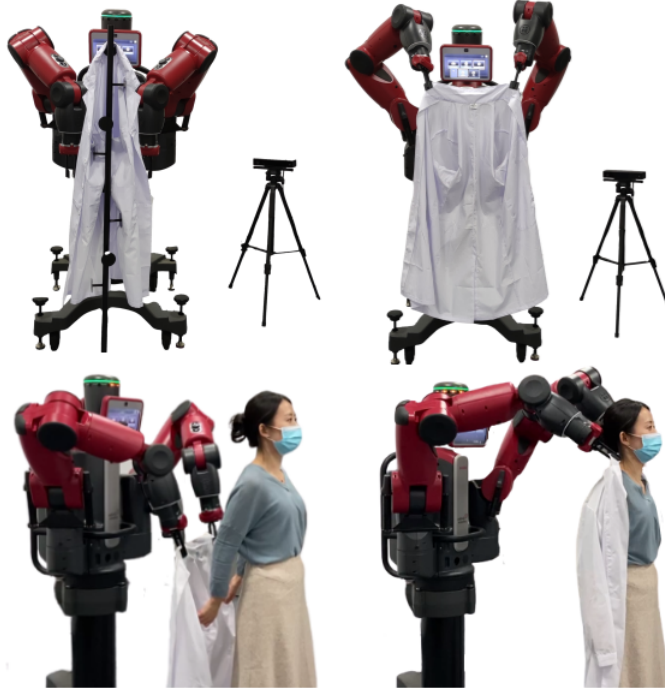
Fig. 1: The Baxter humanoid robot automatically recognizes the hanging clothes’ grasping points and then unfolds the clothes to a wearable state so as to assist users with dressing. The grasping points of the clothes are recognized by our proposed Cross-Domain Representation Learning framework.
