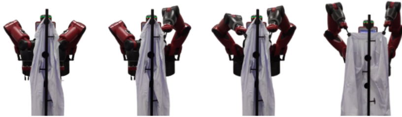
Fig. 6: The entire procedure of unfolding clothes by a Baxter robot. Our CDRL framework calculates the Cartesian coordinate of the clothes grasping points, then the Baxter robot performs motion planning to grasp and unfold the clothes to a wearable state. More detailed video demonstrations can be seen in the supplementary file.
