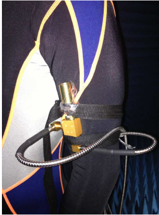
Fig. 1. Scalar horn with an OMT, waveguide-to-coaxial adaptors and coaxial cables, mounted on the arm.
