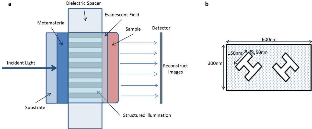
Figure 1. Schematic of: a - the proposed super-resolution microscope; b - the chosen metamaterial unit cell design, two ‘H’ shapes at  $\pm 45^\circ$  to the normal. The metalens is formed from an array ( $100 \times 100 \mu\text{m}$ ) of these unit cells.
