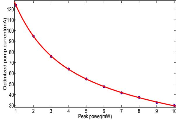
**Fig. 5** Optimized pump current versus peak power  $P_{in}$  .
