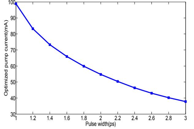
**Fig. 6** Optimized pump current versus input pulse width
