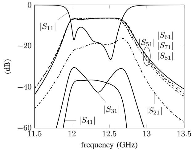
Fig. 5. Magnitude of scattering parameters at port 1
