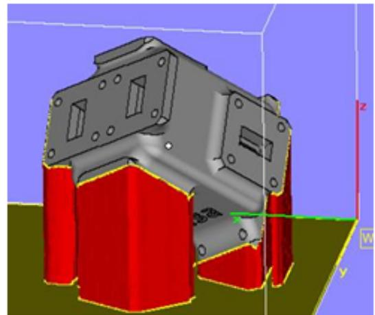
Fig. 3. Geometry placed on material supports in red
