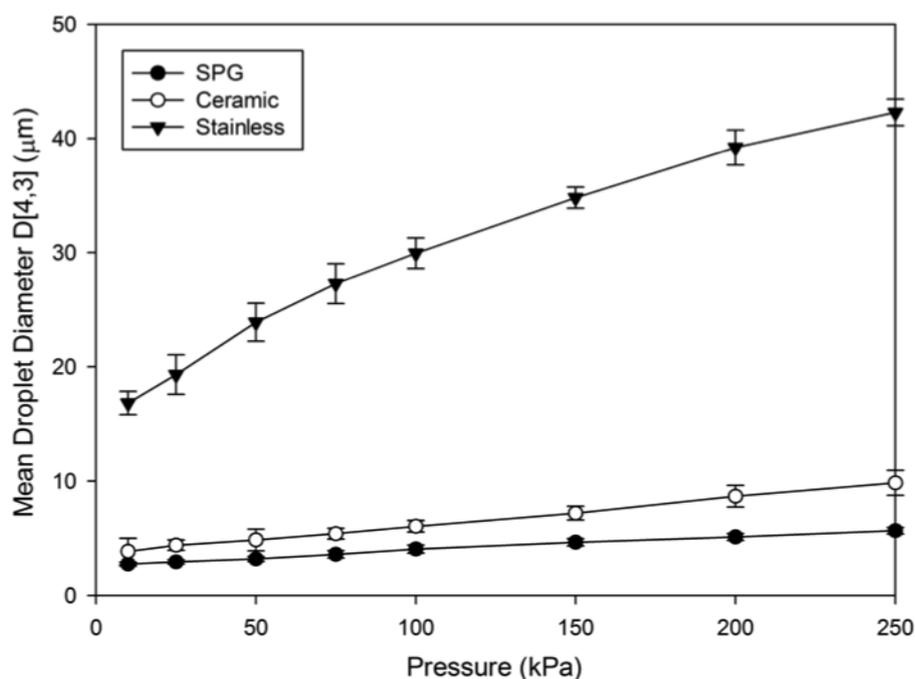
Figure 7. The effects of changing trans-membrane pressure on the droplet size of emulsions produced using the rotating membrane system at 1000 rpm, 1% tween 20 at 1% oil phase volume.
