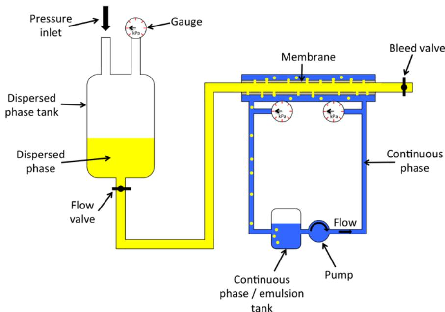
Figure 2. The cross-flow membrane emulsification system used in this study was setup as shown. The membrane module houses the interchangeable membranes such that they separate the dispersed and continuous phases, with the continuous phase flowing along the outside of the membrane tube.
