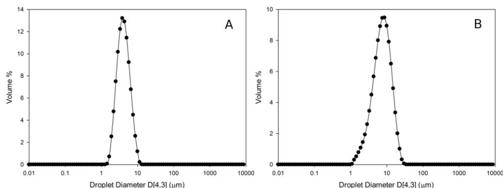
Figure 8a and 8b. A shows the droplet size distribution at 10 kPa 1000 rpm with 1% oil phase volume and 1% Tween 20 as the emulsifier with a 1 $\mu$ m ceramic membrane, and b shows the same emulsion produced at 200 kPa. The relative span of a is 1.13 and of b is 1.54.
