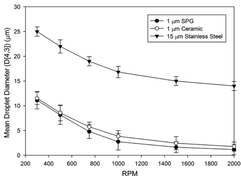
Figure 6. The effects on droplet size of changes in rotation rate (and therefore shear rate) with different membrane morphologies. 1% tween 20 was used to produce emulsions at 1% oil phase volume.
