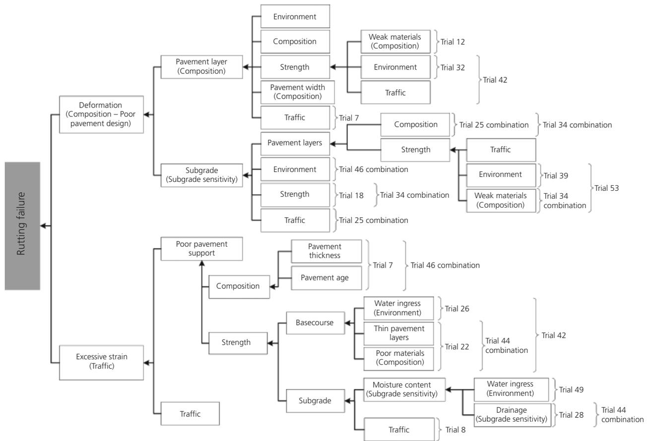
Figure 1. Rutting failure chart with the associated causes of failure identified in the methodology
