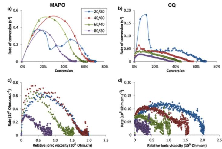
**Fig. 6** Rates of change as a function of conversion or ionic viscosity for the polymerization of MAPO and CQ-composites (note the different vertical scales). Analysis was carried out with FT-NIRS (a and b) or DEA (c and d). The curves show an average of three repeat measurements. The resin composition is indicated by BisGMA/TegDMA in mol%.
