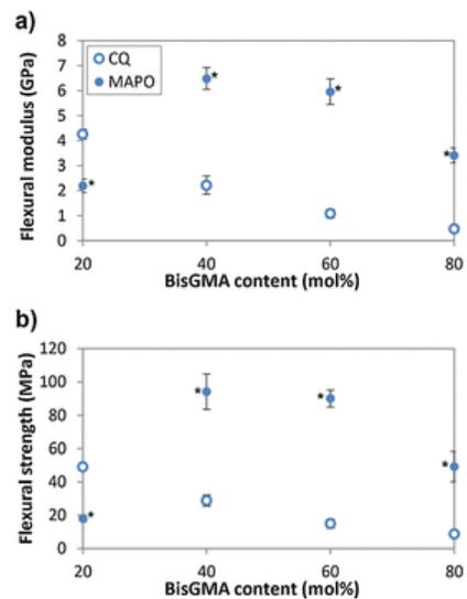
**Fig. 10** (a) Flexural modulus and (b) flexural strength for MAPO and CQ-composites following a one week incubation in 75/25 vol% ethanol/water solution (filled and empty circles, respectively). \* Symbols indicate a significant difference ( $p < 0.05$ ) between the MAPO and CQ series, for one resin composition.
