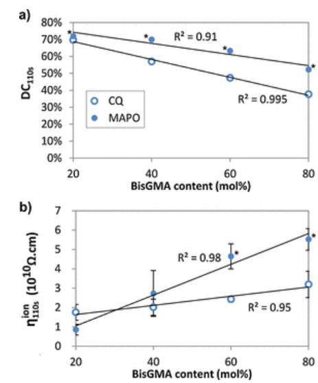
**Fig. 4** a) conversion and (a) Conversion and (b) ionic viscosity values after 110 s of monitoring for MAPO and CQ-composites as a function of BisGMA content.  $R^2$  are the coefficients of determination for the linear regressions. Error bars correspond to standard deviations (symbols may hide the error bars). \* Symbols indicate a significant difference ( $p < 0.05$ ) between the MAPO and CQ series, for one resin composition.
