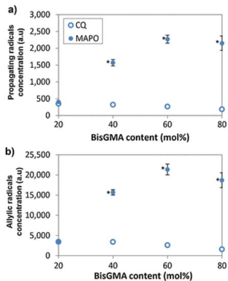
Fig. 8 Trapped radicals concentration in CQ and MAPO-composites (empty and filled circles, respectively). Radical concentration determined 1 h following irradiation. \* Symbols indicate a significant difference ( $p < 0.05$ ) between the MAPO and CQ series, for one resin composition.
