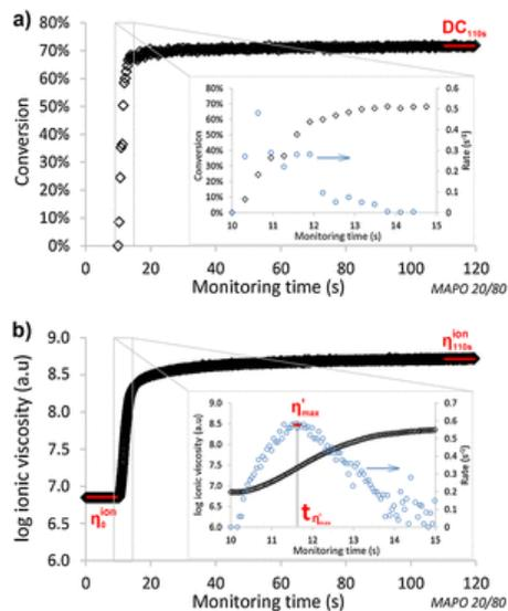
**Fig. 1** Conversion and ionic viscosity as a function of monitoring time for MAPO 20/80 followed by FT-NIRS and DEA, respectively. The data was independently measured and show one sample only. The calculated variables are highlighted in red. Depending on the method and due to varying sampling rates, the determination of rates of signal change could not always be carried out (for example in a).
