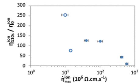
**Fig. 7** Ionic viscosity at 110 s divided by initial ionic viscosity as a function of maximum rate of change in ionic viscosity ( $\frac{\eta_{110s}^{ion}}{\eta_{max}^{ion}}$ ), for CQ and MAPO-composites (empty and filled circles respectively). Error bars indicate standard deviations.
