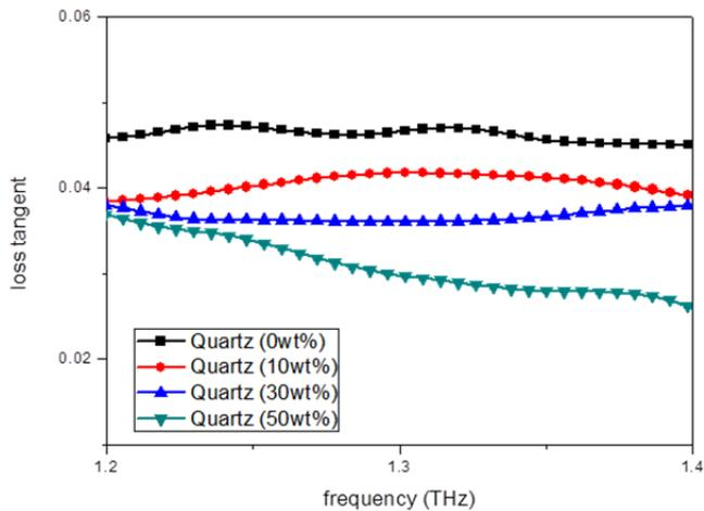
**Fig. 3** Measured loss of the fabricated composite photoresist.
