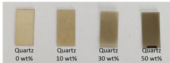
**Fig. 1** *Optical photograph of the fabricated composite photoresist.*
