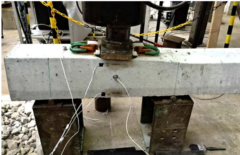
Fig. 3. Arrangement at the rail seat for positive bending test.
