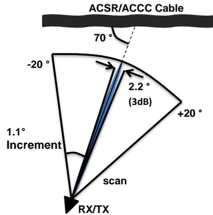
Figure 5. Scenario 2 in overhead power cable imaging experiments
