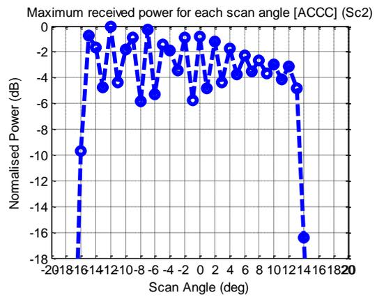
Figure 10. The maximum power in simulations for each scan angle [ACCC] (Scenario 2)
