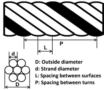
Figure 2. Physical parameters of a helically wound cable
