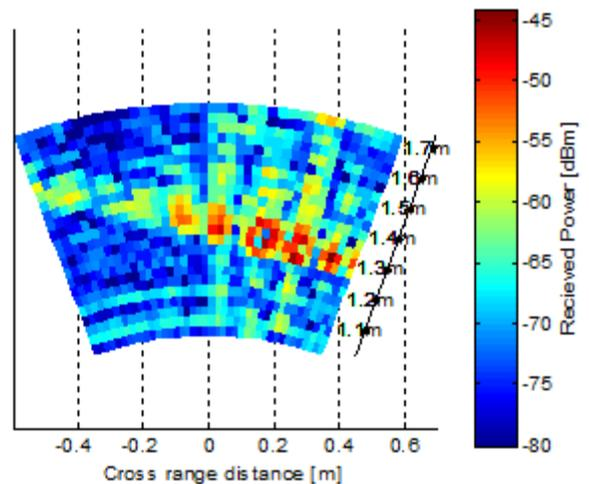
Figure 12. Image obtained by imaging ACSR cable [scenario 2]
