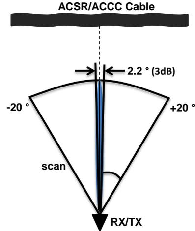
Figure 4. Scenario 1 in overhead power cable imaging experiments
