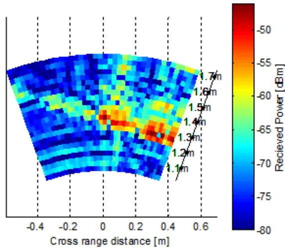
Figure 14. Image obtained by imaging ACCC cable [scenario 2]
