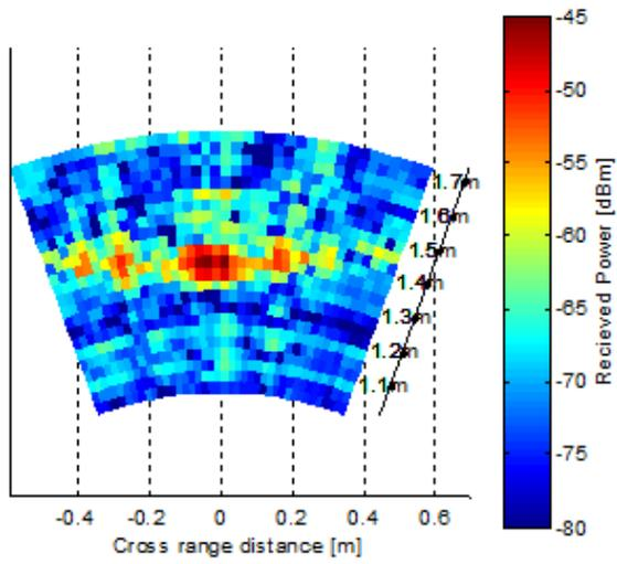
Figure 13. Image obtained by imaging ACCC cable [scenario 1]
