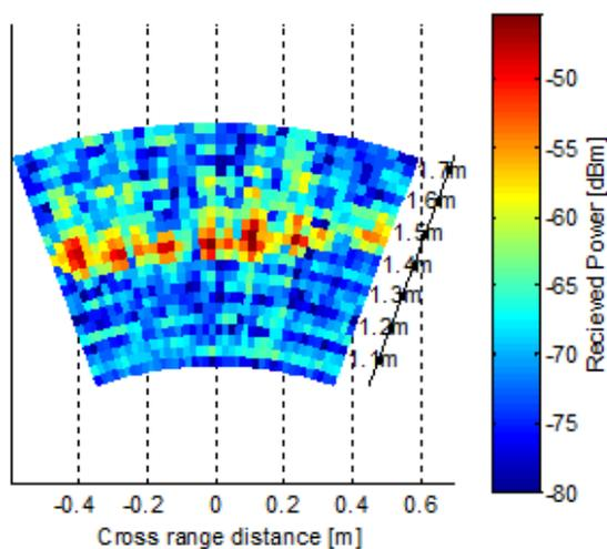
Figure 11. Image obtained by imaging ACSR cable [scenario 1]
