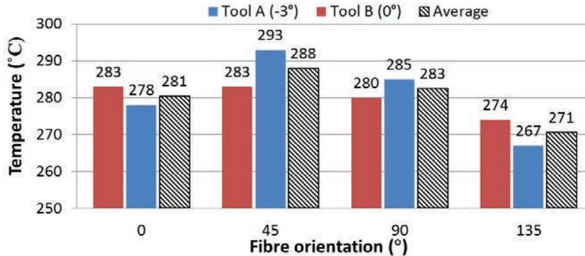
Fig. 7. Temperatures measured when slotting unidirectional laminates.
