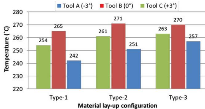
Fig. 6. Temperatures measured when slotting Type-1, Type-2 and Type-3 MD laminates with different routers.
