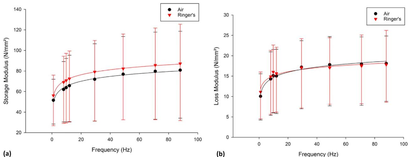
Fig. 1. Frequency-dependent viscoelastic properties, (a) storage and (b) loss modulus ( $N/mm^2$ ), of articular cartilage tested in air and in Ringer's solution (median  $\pm$  95% confidence intervals,  $n = 3$ ) with natural logarithmic regression trendlines). In total 8 specimens from 3 femoral heads were tested.
