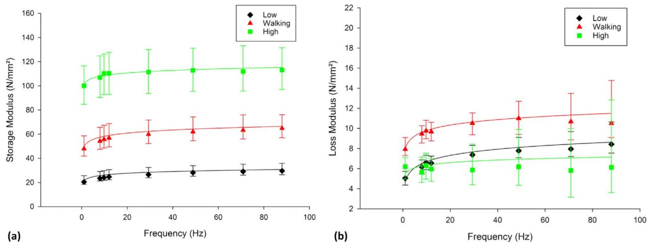
Fig. 2. Frequency-dependent viscoelastic properties, (a) storage and (b) loss modulus ( $N/mm^2$ ), of articular cartilage tested at low, normal walking and high stress ranges (median  $\pm$  95% confidence intervals,  $n = 8$ ) with natural logarithmic regression trendlines). In total 8 specimens from 8 humeral heads were tested in air.
