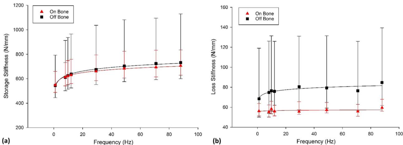
**Fig. 5.** Frequency-dependent viscoelastic properties, (a) storage and (b) loss stiffness (N/mm), of articular cartilage on bone and off bone (median  $\pm$  95% confidence intervals, [n = 8] with logarithmic regression trendlines). In total 8 specimens from 8 humeral heads were tested.
