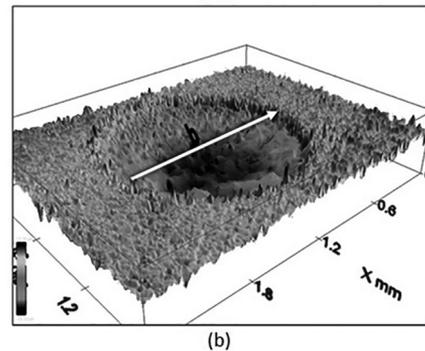
**Figure 1.** Wear coefficients of steels after quenching at 900 °C and quenching at 900 °C plus tempering at 600 °C (a) and wear crater in the specimen surface of the steel (b). The arrow indicates the crater size after the test (COM).
