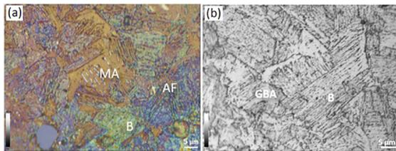
**Figure 3.** 0.08 Nb steel: the first shows the microstructure after quenched at 900 °C (Lepera - COM). The second shows the microstructure after quenched at 900 °C and tempered at 600 °C (Nital 2% - COM).
