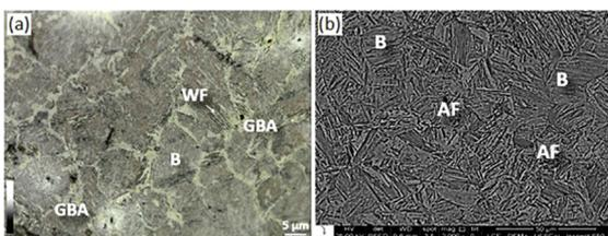
**Figure 4.** 0.01 Nb steel: the first shows the microstructure after quenched at 900 °C (Nital 2% - COM). The second shows the microstructure after quenched at 900 °C and tempered at 600 °C (Nital 2% - MEV).
