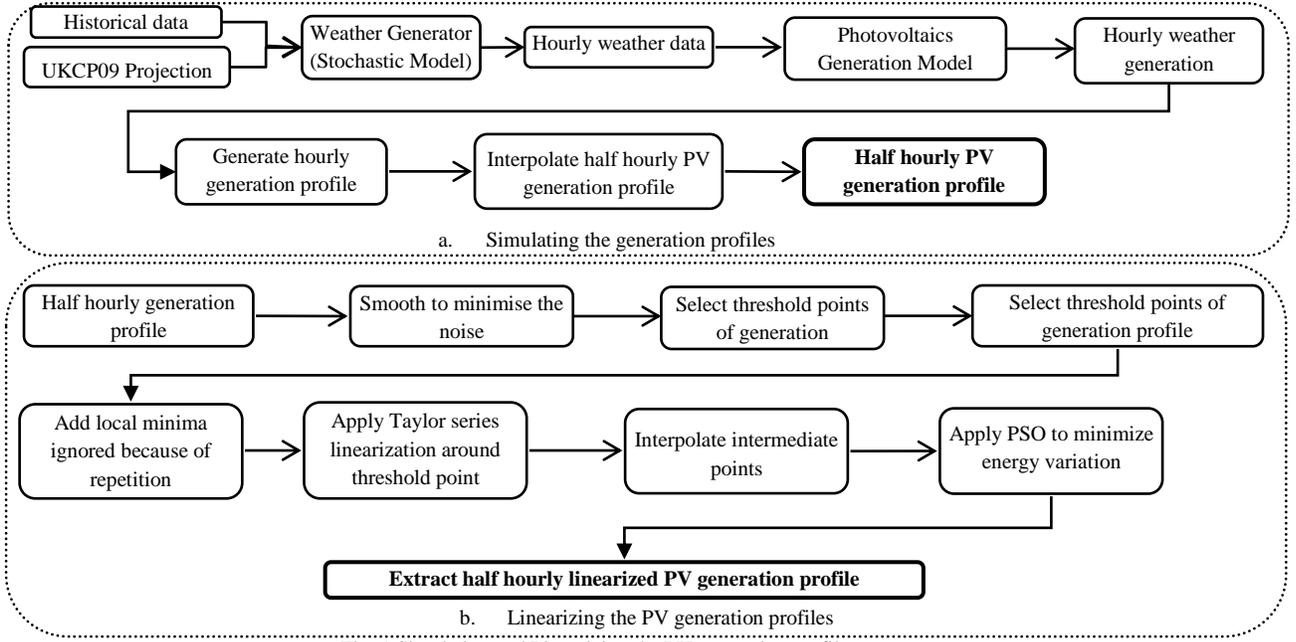
Fig. 1 Simulating and Linearizing the PV generation profile
