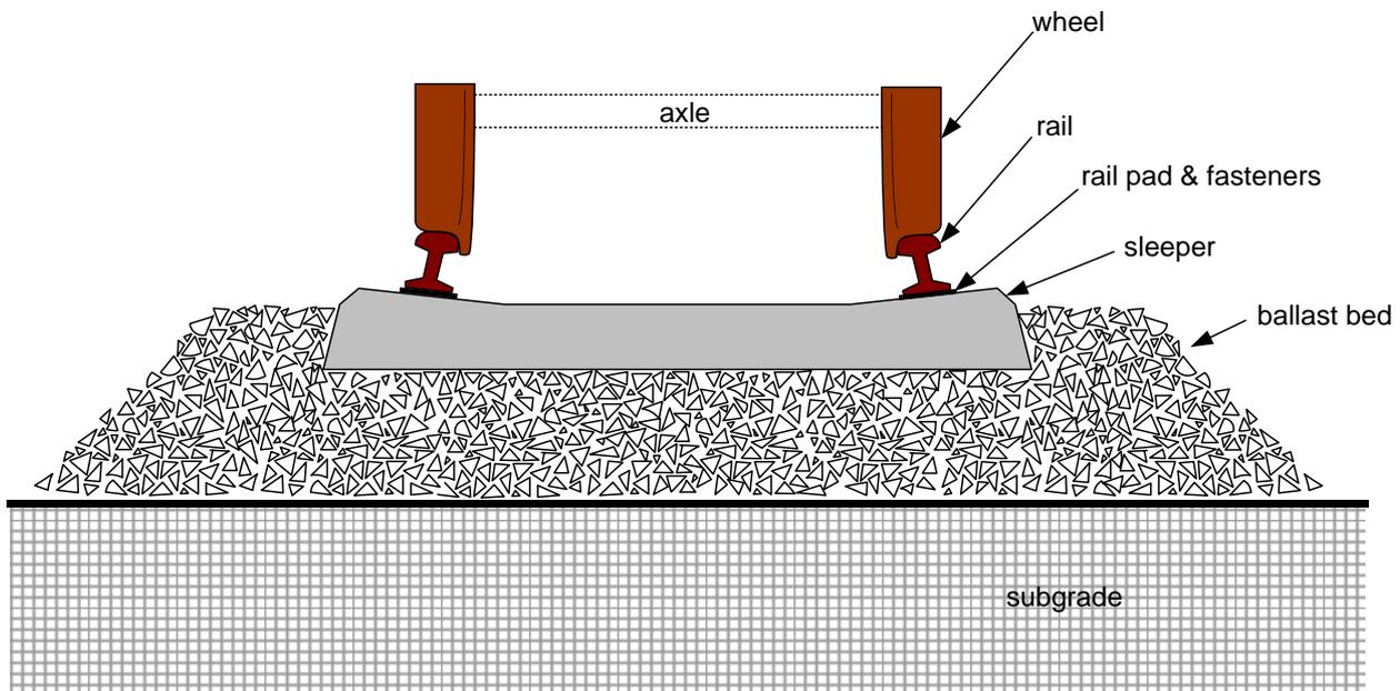
Figure 1: Typical ballasted railway track components.
