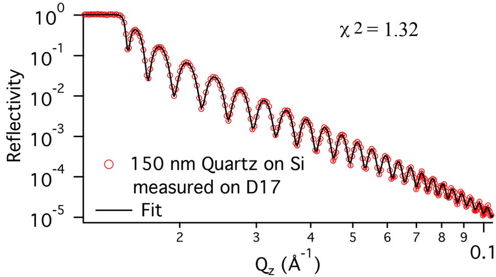
Fig. 4. NR versus  $Q_z$  (both on  $\log_{10}$  scale) from a 150 nm thick quartz film on silicon, measured on D17 using three angles:  $0.8^\circ$ ,  $3.2^\circ$  and  $6.2^\circ$  using a wavelength range from 2.5 – 25 Å. The angular resolution was 0.8% (FWHM) and the wavelength resolution varied from 0.9 – 1.4%. The beam footprint was  $3 \times 5 \text{ cm}^2$ . Note that only the low  $Q_z$  part of the reflectivity curve is shown, whereas the fit covers the whole momentum transfer range.
