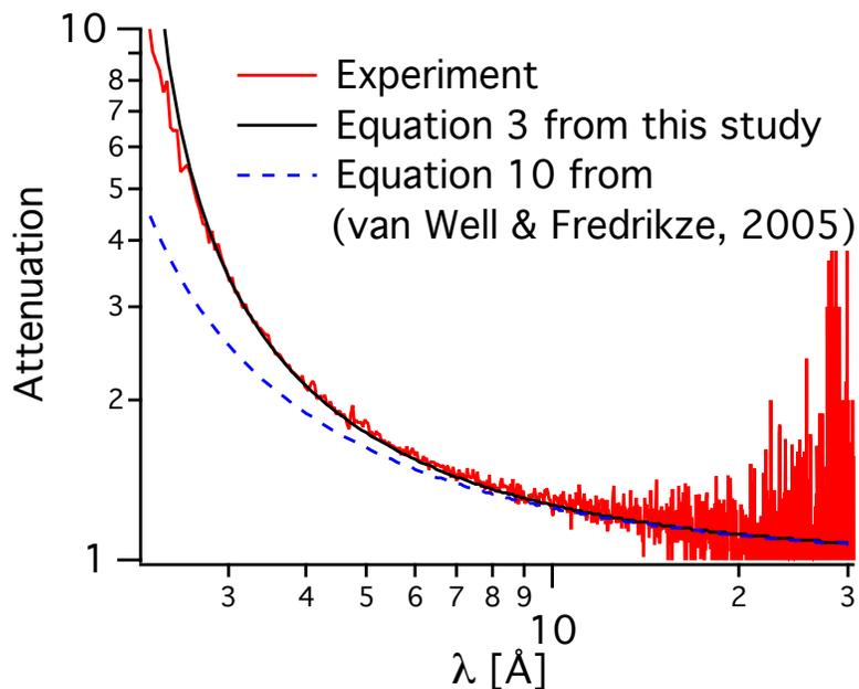
Fig. 3. The red curve shows the measured transmission on D17 of a white beam at zero opening angle  $\phi$  divided by the transmission at a chopper opening of  $-0.26^\circ$  versus wavelength. The black solid curve is the theoretical result using eq. 3 and the broken line is obtained by using eq. 10 from (van Well & Fredrikze, 2005). Both axis are on  $\log_{10}$  scale.
