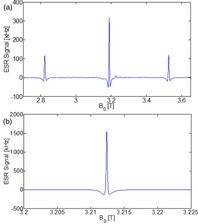
Fig. 5. ESR experiments performed with the 92 GHz single-chip detector. (a) ESR spectra of a  $50 \times 50 \times 40 \mu\text{m}^3$  sample of ruby (see text) with  $\nu_m = 9.8$  kHz,  $B_m = 0.15$  mT,  $B_1 \cong 0.3$  mT,  $\Delta f = 0.25$  Hz,  $t_s = 18$  min,  $T = 200$  K; (b) ESR spectra of a  $3 \times 3 \times 3 \mu\text{m}^3$  of BDPA (see text) with  $\nu_m = 98$  kHz,  $B_m = 0.12$  mT,  $B_1 \cong 0.25$  mT,  $\Delta f = 0.25$  Hz,  $t_s = 4.5$  min,  $T = 200$  K.
