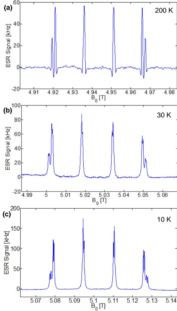
Fig. 6. ESR experiments performed with the 146 GHz single-chip detector. (a-c) ESR spectra of a  $40 \times 40 \times 5 \mu\text{m}^3$  sample of 1%  $\text{Cu(II)(mnt)}_2$  in  $\text{Ni(mnt)}_2$  with  $\nu_m = 98 \text{ kHz}$ ,  $B_m = 0.15 \text{ mT}$ ,  $B_1 \cong 0.6 \text{ mT}$ ,  $\Delta f = 0.25 \text{ Hz}$ ,  $t_s = 16 \text{ min}$  at (a) 200 K; (b) 30 K; (c) 10 K.
