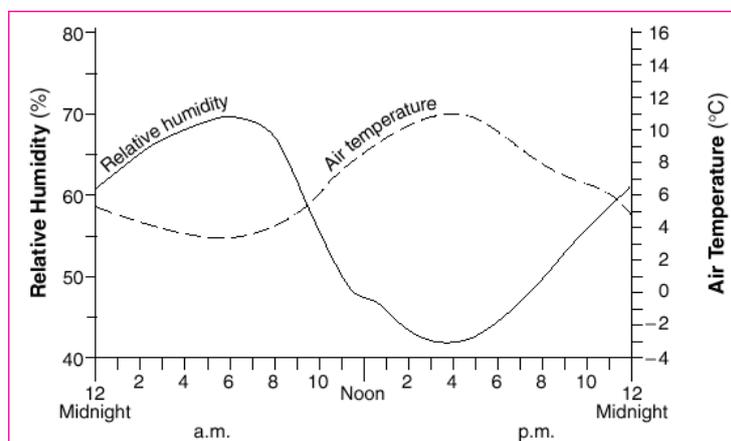
Figure 10. Relationship between relative humidity and temperature.
