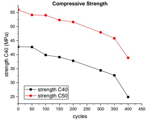
(b) Concrete strength C40 and C50 (400 cycles)
