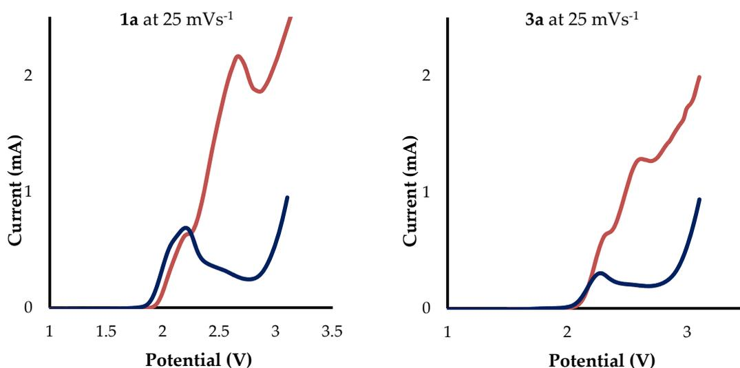
**Figure 3.** Linear sweep voltammetric oxidative response from surveying the scan rate of **1a** and **3a**. Conditions: MeCN/MeOH or H<sub>2</sub>O (10:1), 500 mM Bu<sub>4</sub>NClO<sub>4</sub>, 22.0 mM of analyte, W.E. = GC, C.E. = Pt wire, R.E. = Ag<sup>+</sup>/Ag (-0.057 V versus Fc<sup>+</sup>/Fc),  $\nu$  = 5-250 mVs<sup>-1</sup>. Data for  $\nu$  = 25 mVs<sup>-1</sup> shown for clarity.† Solvent system: **Red** = MeCN/MeOH, **Blue** = MeCN/H<sub>2</sub>O.
