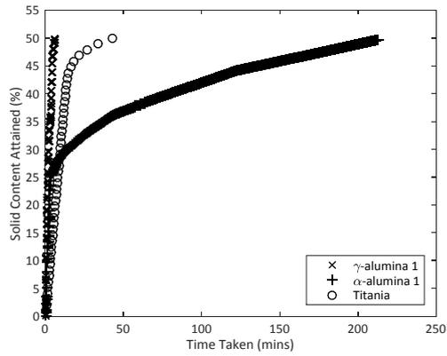
Figure 9: Slurryability approach 1 – time taken to prepare a 50 wt% slurry
