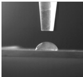
Figure 4: Example sessile drop sat on a powder bed
