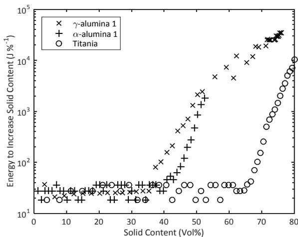
Figure 13: Energy to increase the solid content slurry by 1 wt% against the slurry solid volume concentration
