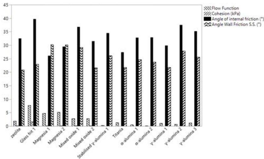
Figure 6: Shear cell measurements for initial 13 powders
