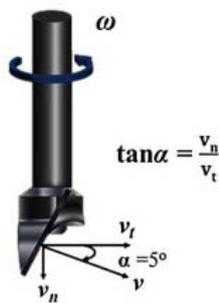
Figure 3: Freeman FT4 powder rheometer helical impeller blade used for conditioning and measurement
