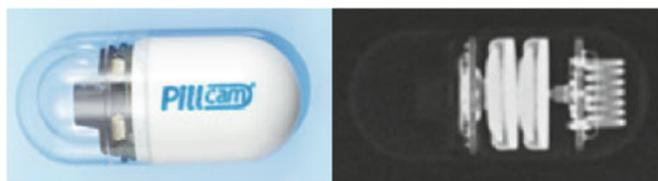
Fig. 1. Configuration of Pillcam SB with internal helix antenna [1].
