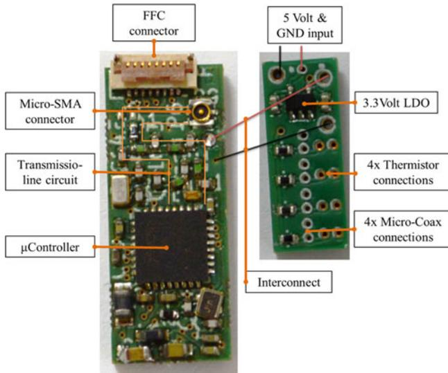
Fig. 4. (Left) RF board and (right) thermistor board.
