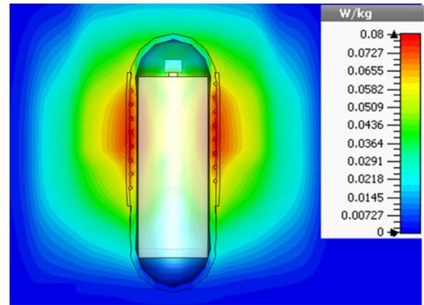
Fig. 11. SAR distribution of the simulated antenna system.
