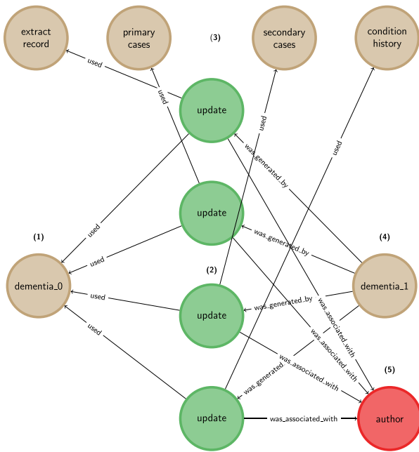
Figure 3: An example data provenance trace showing an update to a dementia phenotype, using the W3C PROV standard. The initial version of the phenotype (1) is updated by four edit activities (2), each of which modifies a component of the definition (e.g., record extract logic, diagnostic codes, previous history) (3), in order to generate a new version (4), and the process is linked with the author making these edits (5).
