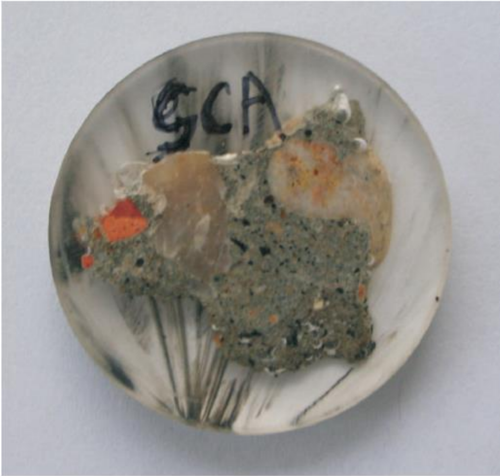
Figure 13 Concrete particle sample for XRD testing
