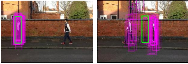
a) Frame 1 b) Frame 55. After cross-over Fig. 2. Failure modes in environmental clutter
