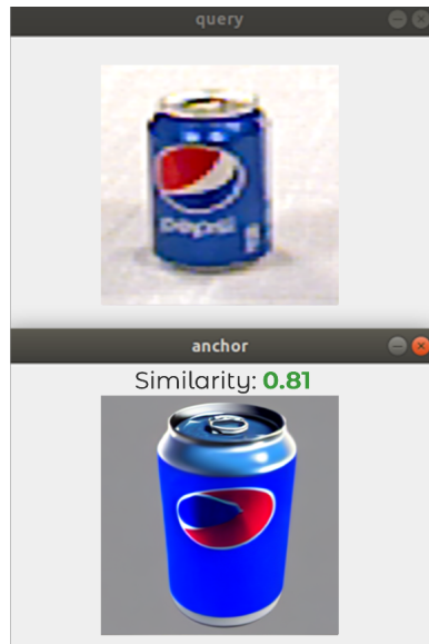
Fig. 11: A comparison of the real vs. imagined object, top: actual robot camera input; bottom: extracted imagined object.
