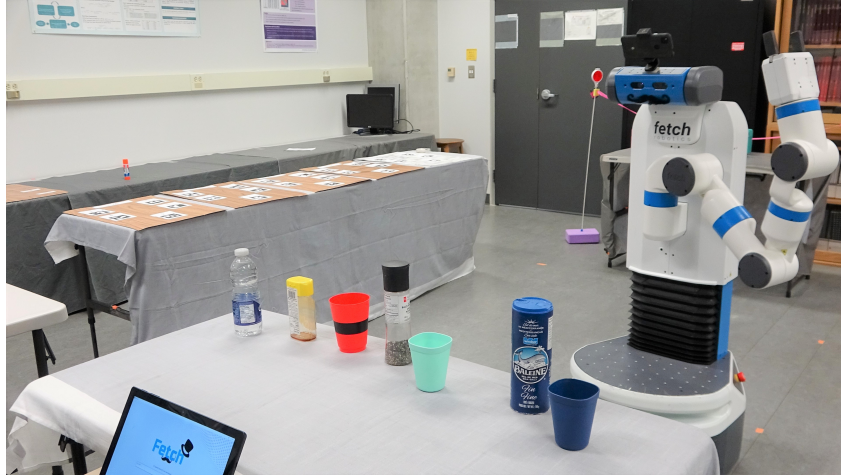
Fig. 13: Experiment setup and the Fetch Robot.
