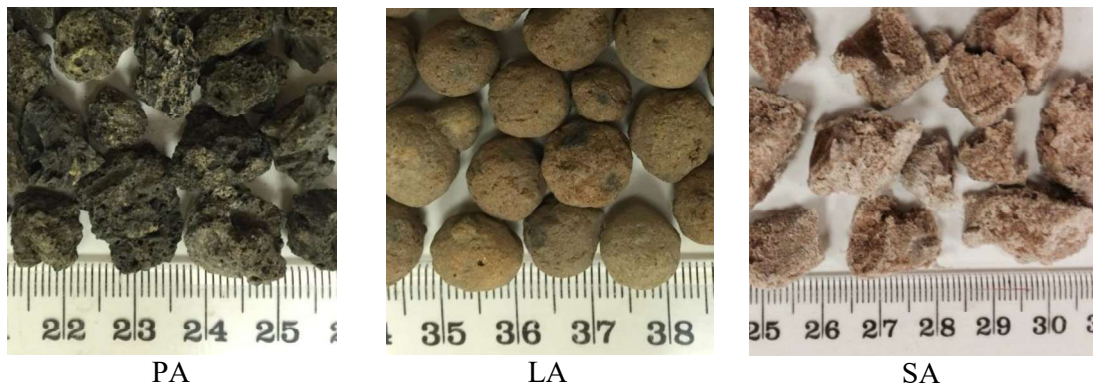
140 Figure 1: Various types of coarse aggregate used in this study: PA; LA; and SA
