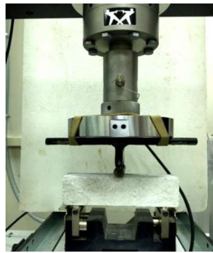
212 Figure 5: Failure deformation test setup using INSTRON machine
