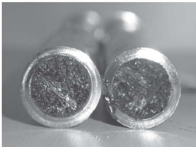
Fig. 9— Photograph of cross section of catalyst bed showing coke deposition on and around CoMo pellets at 475°C.
