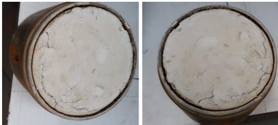
Figure 4 Typical compacted soil specimen after 3 days of drying at 40°C
