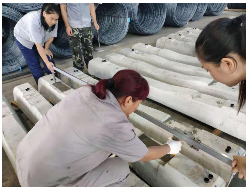
Figure 9. Sleeper critical dimension measurement
