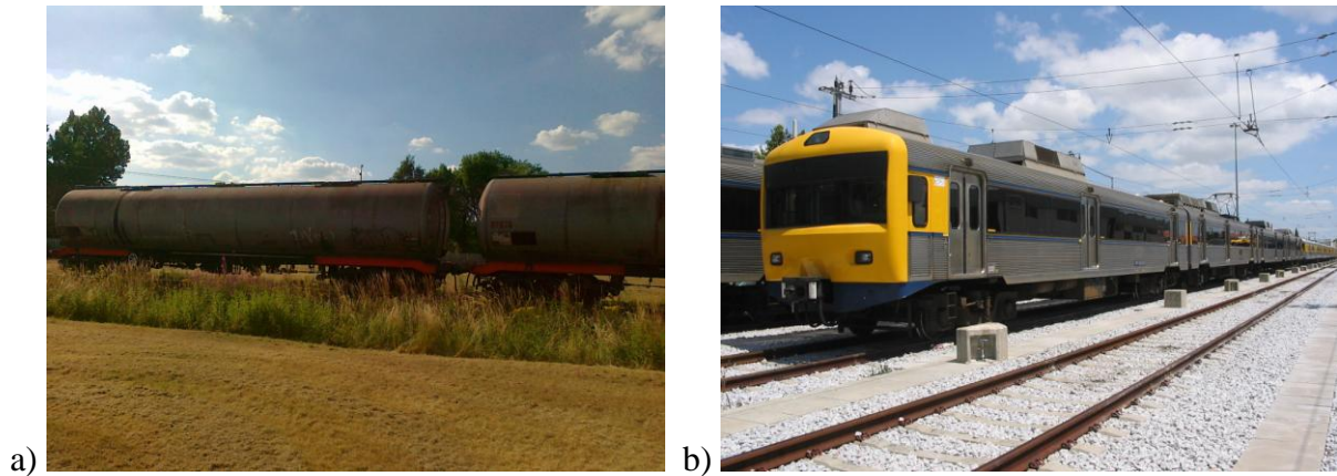
Figure 5: a) Tanker freight wagons with several axle bearings artificially damaged in the roller or race using a power tool, b) EMU with one defective wheel (tread shelling) used for experiments in Portugal.
