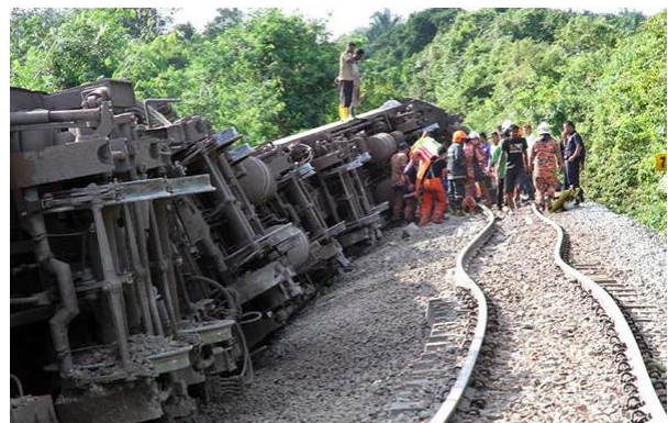
Fig. 2: KTMB train derailed due to rail buckling and had landed on its side, trapping the driver and injuring about five passengers just before the Kempas, Johor station southern part of Malaysia.
