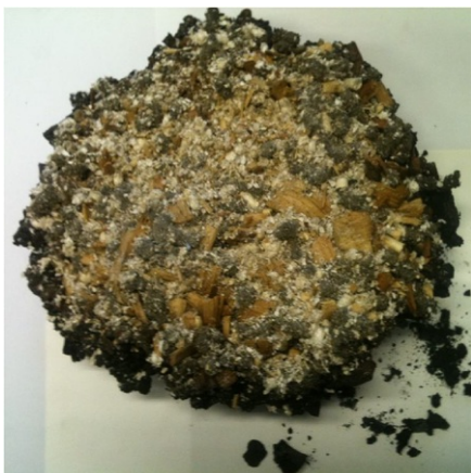
Fig. 3 Agglomerations formation of co-form® rejects in a gasifier [12].
