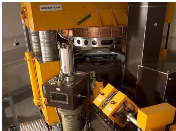
Figure 3: The MC40 Cyclotron, photographed during the opening ceremony in Birmingham: the upper yoke is raised to show the internals.
